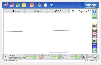
The rate deviation is recorded continuously on the screen. During the measurement rate, amplitude and beat error are displayed numerically.
