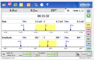
The Vario mode measures the stability rate, amplitude and beat error over a longer period. This clear display mode is an ideal complement for a rapid or prolonged control (up to 100 hours).
