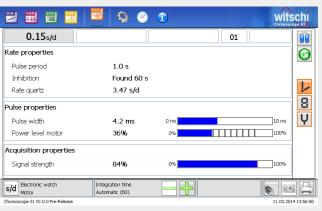
Together with the optional "Quartz Microphone" transducer for electronic watches, large numbers of electronic watches can be measured with a non-contact system. In the case of analogue quartz watches, the current rate, inhibition period, corrected rate, power level and pulse width of the motor are measured. The current rate can be specified in the case of watches with a liquid crystal display and tuning fork watches.
