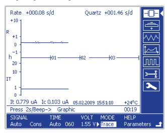
The Trace mode allows a long range diagram recording of the rate deviation and the chopping level. Thereby are determined changes in the rate deviation (e.g. caused by temperature variations) as well as changes in the chopping level of watches with adaptive motor pulses (e.g. caused by a change of date) for a duration reaching 60 h.
