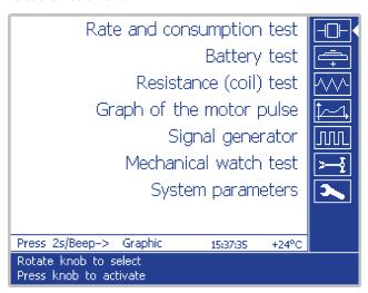
The operation is simple and easy to understand. Ordinary standard measurements can be largely automated. The instrument determines the associated parameters. For more advanced users, measuring parameters can also be manually selected according to requirements. The results, menus and parameters appear on the ¼ VGA LCD graphic display.
