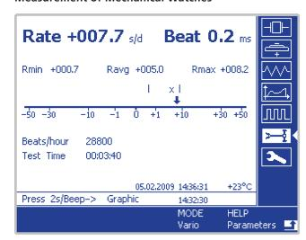
The VARIO display mode provides a clear-cut and efficient measurement of the rate and the evaluation of the rate stability. The results are displayed in graphical form on a logarithmic scale..
