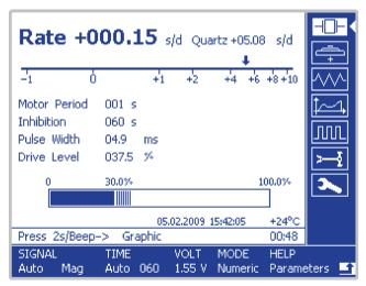
Along with the display of the rate accuracy, the analysis of the magnetic signal can provide the period and the pulse width as well as the inhibition period and the chopping level. With this information, it is possible to determine the efficiency of a watch drive with asservissement.
