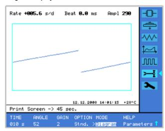
The diagram is continuously drawn. The numerical rate, amplitude and beat measurements are displayed at the end of the first measuring time. The average of the single measurements is updated every 2 seconds, even with a longer set measuring time.
