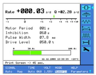
The analysis of the magnetic signal provides a display of the accuracy. It also allows checking the period duration, the pulse width as well as the inhibition period and the drive level. Based on this information, it is possible to determine the efficiency of a watch drive without opening the watch.
