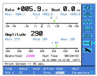
This mode provides a clear-cut assessment of the rate and amplitude stability. The results are displayed in graphical form on a logarithmic scale. The min., average and max. values of single measurements since the beginning of the measurement process are displayed under the current results. The beat number as well as the measuring time since the beginning of the measurement process are also displayed.
