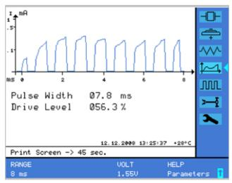
The current pulses are shown as a curve. The pulse shape is an important criterion about the good operation of the watch. Faults can be detected in the mechanical part of the watch by comparing its measurements to those of a watch of the same type in good condition. In addition, the pulse width and the drive level are displayed numerically.
