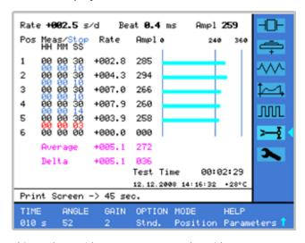
This mode provides measurement cycles with 2 to 6 test positions by manually rotating the microphone. The instantaneous measurements of rate, beat and amplitude are collected during the measurement process. The average of the rate and amplitude for each test position is displayed at the end of the measurement cycle. The measured values of the amplitudes are also represented by a light blue bar.
