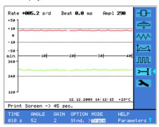
In this mode, the measurement result of rate and amplitude are recorded graphically in a time range depending on the measuring time. It can be selected from 8 minutes to max. 64 hours. This provides a way to detect and locate recurring deviations (e.g. faults in the gear train).
