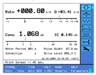
The watch to be tested is supplied with a variable voltage. Moveable probes are used as contact elements. The hands can be observed during measurement by means of the built-in mirror.
