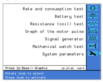
Largely automated measurement sequences provided by the instrument result in an unmatched user-friendliness. For more advanced users, measurement parameters can also be manually selected according to requirements. The main menu, results, parameters, submenus and information are presented on a colour display.
