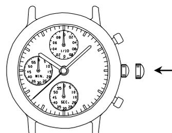
3.Push the crown back in to the normal position in accordance with a time signal.
