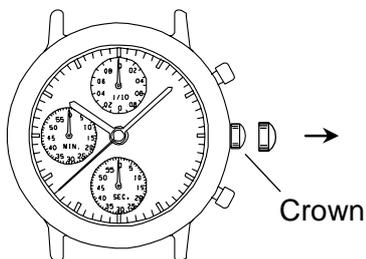
1.Pull out the crown when the second hand is at the 12 o'clock position. The second hand will stop on the spot.
