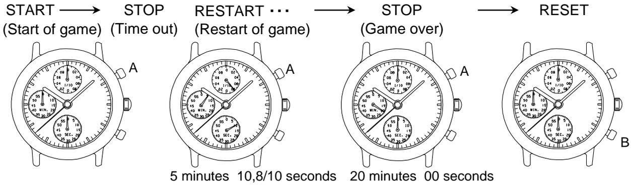
\*Restart and stop of the stopwatch can be repeated as many times as necessary by pressing button A
