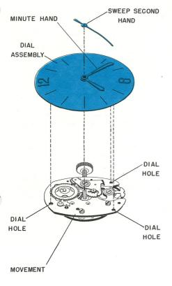
a) Remove sweep second hand. Do not remove the minute or hour hand.
