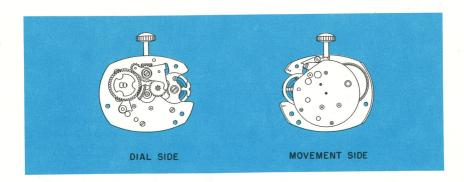
The TIMEX Model 24 is an 111/4"'x91/4" movement featuring "V-conic" bearings system and rugged two plate design. The TIMEX Model 24 movement is readily distinguished from other TIMEX models by the round movement plate.
