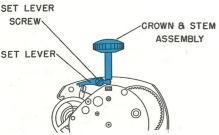
To remove the crown and stem assembly, invert the movement so that the movement plate is facing you. Turn the set lever screw approximately one turn and lift the tail of the set lever out of engagement with the stem. The crown and stem can now be removed.
