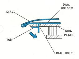
c) Once the dial is off the movement, there is no need for further disassembly of the dial assembly for cleaning unless severe contamination is present on the friction and cannon pinions. Should further disassembly be necessary, removal of the minute hand will free the friction and cannon pinion assembly. The friction pinion is held in the cannon pinion by a snap fit.
