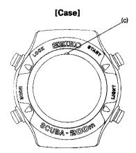
· Align the protrusion (C) on the face side of the panel cover with the notch (c) inside the case.
