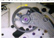
Using sturdy tweezers, push the stud outward from the direction of the arrow shown in the illustration until it is removed from the stud support.
