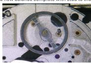
2. Set the balance bridge and tighten the balance bridge
