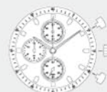
OS30 height 4.13mm chrono hour/min/sec 3 year battery life (SR927W)
