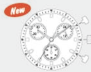
JS00 height 4.18mm stopwatch 30min/sec, 24 hour 2 year battery life (SR621SW)
