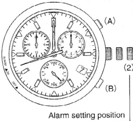
1. Turn the crown and set the mode hand to the alarm (ALM) position.
