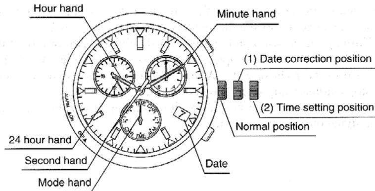
2. When the crown is pulled out to position 2(time setting position), the second hand rapidly advances to the 6 seconds position and stops.
