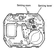
Remove the setting stem while pushing the setting lever at the site indicated by the arrow using a fine instrument like tweezers, etc. The above procedure should be carried out with the setting stem remaining in its normal position.
