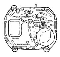
When mounting the supporter for plate complete, make sure that three points of the supporter for plate complete which are circled in the diagram have been placed within the LC display panel supporter.
