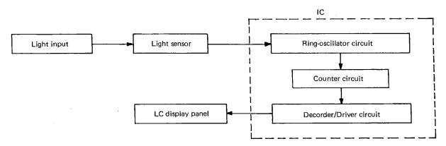
The light input to the watch is converted to the voltage corresponding to the strength of the input light through a light sensor. The ring-oscillator circuit oscillates at a frequency (F) corresponding to the input voltage. This frequency is counted by the counter circuit and the counted number if displayed on the LC display panel divided into 20 levels through the decorder/driver circuit.
