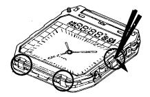
b) For removing the plate complete, placing the watch so as to face its LC display panel downward, the supporter for plate complete at the above-mentioned six hooks as pressing softly the center of the plate complete with finger.
