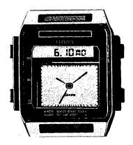
This is an LCD analog/digital display watch provided with a segmented luminous indicator through the light sensor technique.
