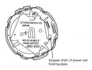
The power cell holding plate is slided left for detachment while the stopper shaft (shown by an arrow in the left diagram) is pushed up light with a tweezers or the like.
