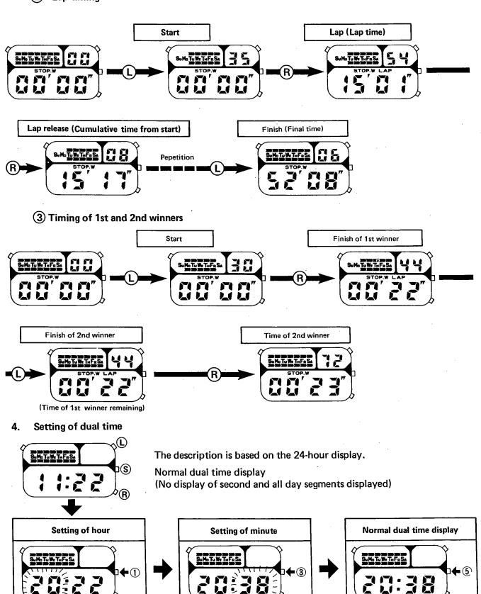
The normal dual time display can be reset at any moment with push of (L) button.
