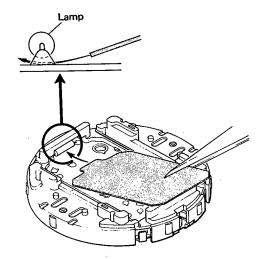
The reflecting plate of this watch slips under the lamp. (This is to enhance the efficiency of the light.) Thus, the reflecting plate has to be put in and out with a slight tilt.
