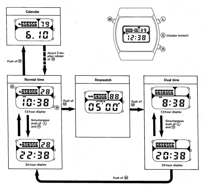
The normal time display is switched to the calendar display with push of  $\bigcirc$  button. And the normal time display is reset in about 2 seconds after release of  $\bigcirc$  button.
