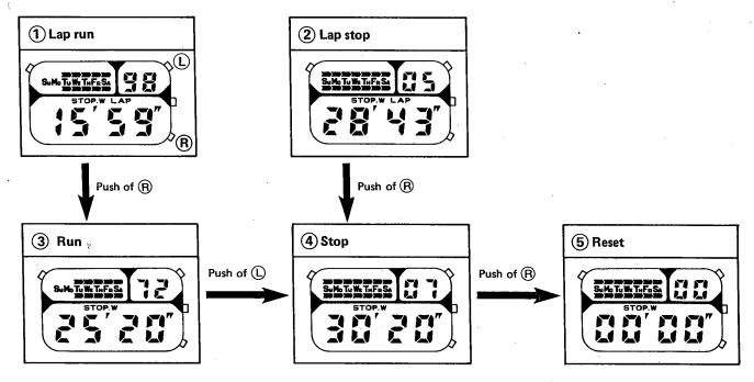
The segment of the day runs from left to right under the run mode (including lap run), and all day segments are displayed under other modes.
