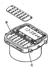
(7) Set the conductor packing, putting the B-part first and then up to the C-part in sequence. In this case, it must be confirmed that the conductor packing never protrudes over the arrow-marked surface of the packing holder. (It is quite all right even though the center area of the conductor packing may swell up a little.)
