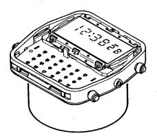
(3) The movement is set in, making sure the packing for movement rest never protrudes over the back side of the caseback.
