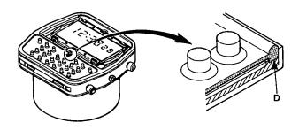
(8) Put on the packing (grey), first matching the groove at the D-part with the packing (grey) and then setting the packing (grey) along the tip outer circumference of the packing holder in a correct way.
