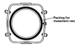
(2) The packing for movement rest must be set accurately to the groove part of the case center body. Be careful not to confuse this packing with that for the caseback since they are in the same size. Avoid applying the silicon oil to the packing.
