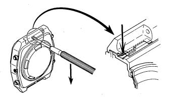
The cross-section of the watchcase appears when the band is removed. And a spring is seen at the cross-section. As illustrated in the diagram, the spring is pushed with a driver to remove the bezel. \*The bezel must be removed at the 12-o'clock direction.
