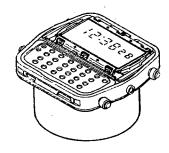
(6) The packing holder rest and the packing holder are put on the rubber spacer. Make sure that the rubber space is never seen through each hole of the packing holder. (If the rubber spacer is seen through the hole, the spacer must be reassembled since is out of position.)
