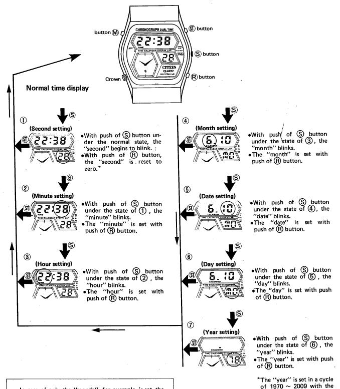
In case of only the "month", for example, is set, the (S) button is pushed four times. Then the "month" begins to blink and can be set with push of (R) button in the necessary pushing frequency. After setting the "month", the (ST) button is pushed
