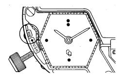
The LC display panel supporter must be set in such a way that the unlocking lever for setting stem is put into the guide hole (with arrow and PUSH marks) of the LC display panel supporter.
