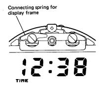
As shown in the left diagram, the connecting spring for display frame is incorporated above the LC display panel holder. It functions to give a contact to the display frame and to prevent the electrostatic "noise" from giving an evil effect to the display.
