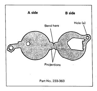
The side 'A' insulates the power cell (-) from the plate complete while the side 'B' insulates the power cell (+) from the power cell connector spring.
