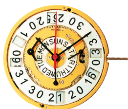
Cal. 5050.C • 4.40 mm Chrono, Day, Big Date 1/10 Second 30 Min. / 12 Hours Small Second
