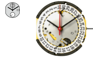
Cal. 3520.D • 4.90 mm Chrono, Date 30 Min. / 12 Hours Small Second
